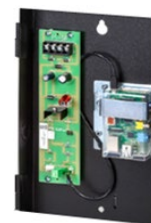
Typical mounting set-up of a SNU module
